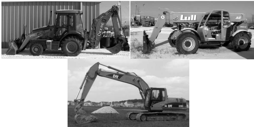
Figure 2.1 Mobile, multi-actuator machines (top left: backhoe loader; top right: telehandler; bottom: excavator)
